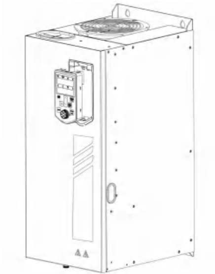
Fig. 3.3-1 Remove and Mount Control Panel
