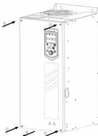
Fig. 3.3-3 Schematic diagram of disassembly and installation of sheet metal housing cover plate
