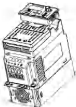
Fig. 3.3-1 Remove and Mount Control Panel
