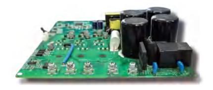
The PV210 series solar pump inverter is a compact and highly integrated professional inverter. It adopts highperformance vect or control technology and is specifically optimized for solar pumping systems. The device integrates precise PID control, higherficiency MPPT (Maximum Power Point Tracking).
